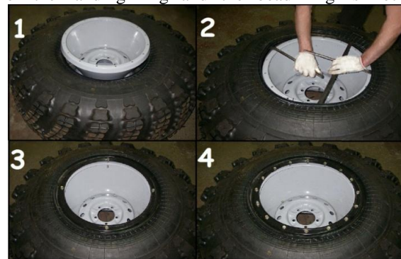
Fig. 10.2. Procedure for mounting the TRECOT tire
