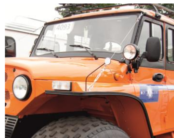
Fig. 20.29 Search lamps with handles, controlled from ATV windows
